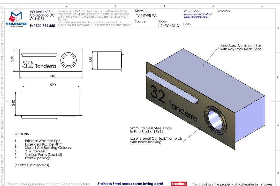
This item is being specially manufactured and may take some time. Please use this drawing to make allowances in your construction to retrofit this item if necessary. To avoid damage to this product it is recommended to fit after construction or at time of rendering.
